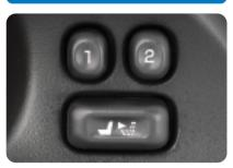
The memory seat controls are located on the driver door. They program and recall driver seat position and outside mirror settings for up to two drivers.
