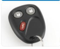
On equipped vehicles, the RKE system locks and unlocks the doors and liftglass from a range of three to 30 feet. At times the range may be shorter than usual, which is normal. If the transmitter does not seem to be working properly:
