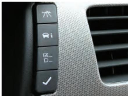
To operate the DIC, the ignition switch must be on. The DIC is controlled through the following four buttons located on the right side of the instrument panel cluster:
