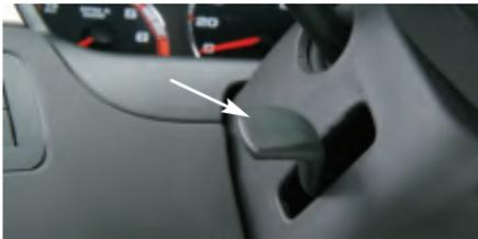
The steering wheel can be adjusted up or down using the tilt wheel lever located on the left side of the steering column.
