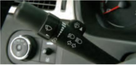
The windshield wipers control is located on the multifunction stalk on the left side of the steering column. It includes the following functions:
