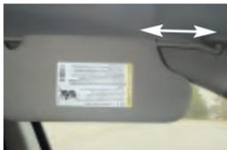
retainer and slid along the rod to cover different areas of the front window and rotated to cover the side window.
