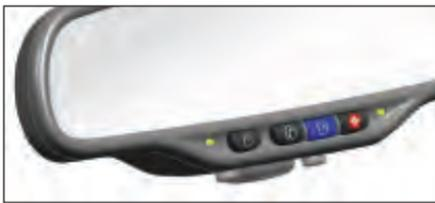
The reading lamps, located on the rearview mirror, can be turned on or off independent of the courtesy lamps by pressing the buttons on the bottom of the mirror, when the doors are closed.
