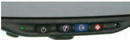
The OnStar system provides in-vehicle safety, security and phone services — available 24 hours a day, 7 days a week — including Advanced Automatic Crash Notification, Automatic Notification of Airbag Deployment and Roadside Assistance. These services are easily accessed through the three OnStar buttons in your vehicle.
