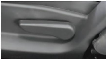
Lift the rear-mounted lever on the outboard side of the seat cushion and move the seatback to the desired position; then release the lever.
