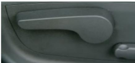
Adjust lumbar support using the front-mounted lever on the outboard side of the seat cushion. Ratchet the lever up to increase support or down to decrease support.
