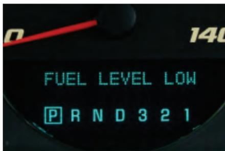
Your vehicle's Driver Information Center (DIC) provides vehicle information, vehicle warning messages and vehicle feature customization. The DIC messages will be shown on your instrument panel cluster display. The DIC display also shows the outside air temperature and compass direction (if equipped).
