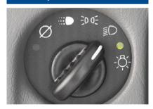
The exterior lamps knob is located on the instrument panel, to the left of the steering wheel.
