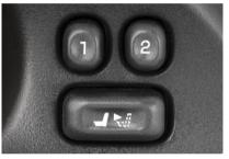
The memory seat controls are located on the driver door. They program and recall driver seat position settings for up to two drivers.
