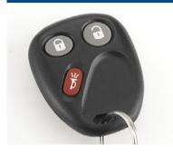
On equipped vehicles, the Remote Keyless Entry (RKE) System locks and unlocks the doors and liftglass from a range of three to 30 feet. At times the range may be shorter than usual, which is normal. If the transmitter does not seem to be working properly:
