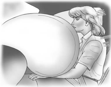
The front outboard passenger frontal airbag is in the passenger side instrument panel.
